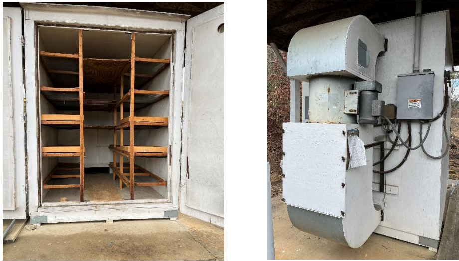
Figure 5. A small hop drier with shelves and forced hot air. Front (left) and back (right). Plans for this drier can be found at https://newcropsorganics.ces.ncsu.edu/wp-content/uploads/2016/11/herb_dryer_leaflet-1.pdf?fwd=no
